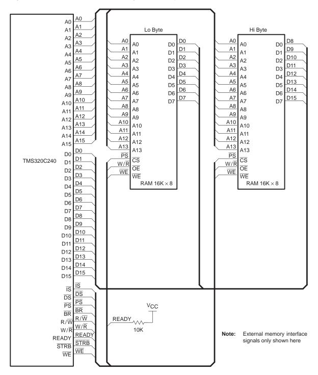
The program select ( $\overline{PS}$ ) signal is connected directly to the chip select ( $\overline{CS}$ ) to select the memory on any external program access. The memory is addressed in any 16K address block in program space. If multiple blocks of memory are to be interfaced in program space, a decode circuit that gates  $\overline{PS}$  and the appropriate address bits can be used to drive the memory block chip selects.
