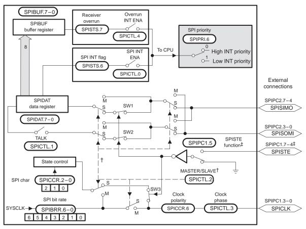
Figure 9–1. 4-Pin SPI Module Block Diagram (Slave Mode)
