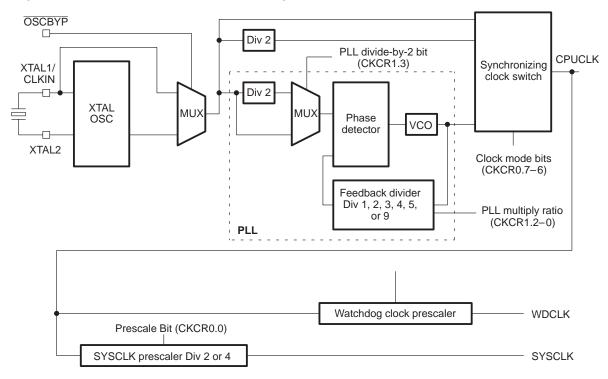
Figure 4–1. PLL Clock Module Block Diagram
