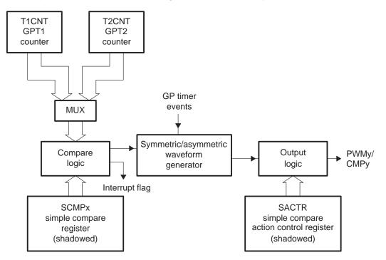
The timing of simple compare outputs is the same as that of the GP timer compare outputs. There is an interrupt flag for each simple compare unit and the setting of these flags is the same as in the GP timer compare operation.
