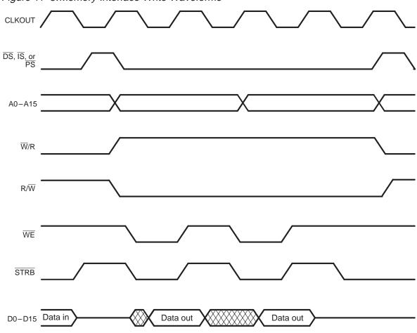
Figure 11–5. Memory Interface Write Waveforms
