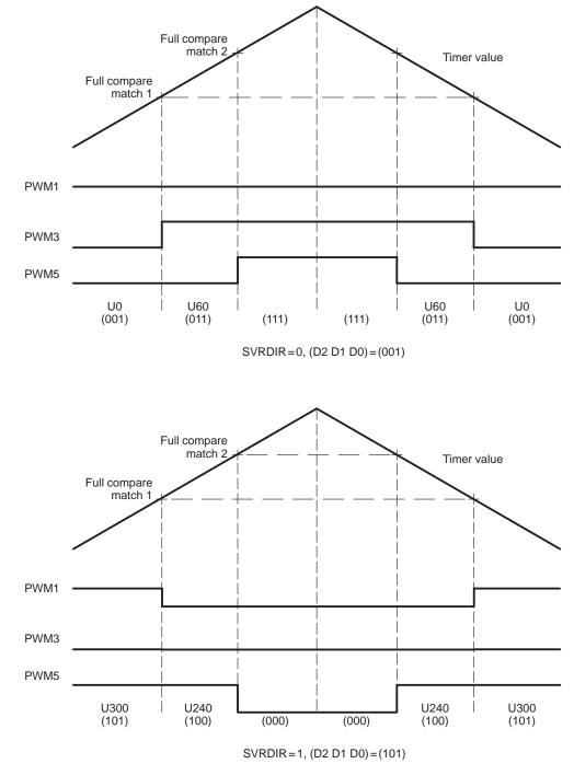
Figure 6–25. Symmetric Space-Vector PWM Waveforms
