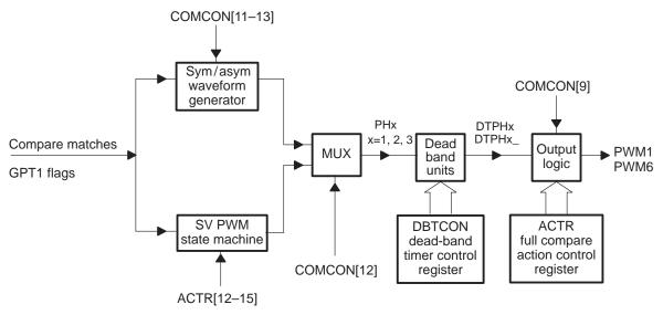
PWM circuits are designed to minimize CPU overhead and user intervention in generating pulse width modulated waveforms used in motor control and motion control applications. PWM generation with full compare units and associated PWM circuits are controlled by the following control registers:
