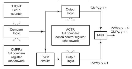
The time base for full compare units and the associated PWM circuits is provided by GP timer 1. This timer can be in any of its six counting modes when the compare operation is enabled. However, no transition happens on compare outputs when GP timer 1 is in the directional up/down counting mode.
