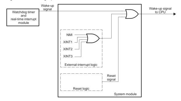
Figure 3–5. Waking Up the Device from Power Down
