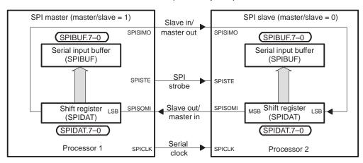
*Figure 9–2. SPI Master/Slave Connection (4-Pin Option)*
