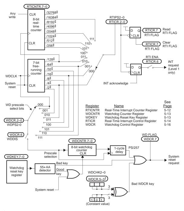
Figure 5–1. Watchdog (WD) and Real-Time Interrupt (RTI) Module Block Diagram
