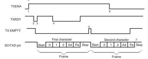
Figure 8-8. SCI TX Signals in Communications Modes
