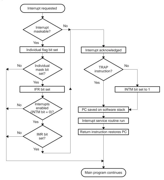
Figure 2–17. Interrupt Operation Flow Chart
