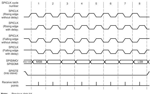
For the SPI, the SPICLK symmetry is retained only when the result of (SPIBRR + 1) is an even value. When (SPIBRR + 1) is an odd value and SPIBRR is greater than 3, the SPICLK becomes asymmetrical. The low pulse of the SPICLK is one SYSCLK longer than the high pulse when the CLOCK POLAR-ITY bit is clear (0) as shown in Figure 9–4. When the CLOCK POLARITY bit is set to 1, the high pulse of the SPICLK is one SYSCLK longer than the low pulse as shown in the same figure.
