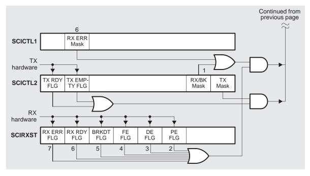
Figure 2–13. Maskable Interrupt Structure for CPU Interrupt Level 1 (Continued)
